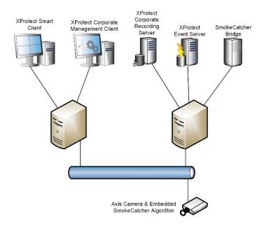
After installation of the SmokeCatcher system, it is required to also configure XProtect to properly handle the incoming metadata. This configuration requires the installation of the MIP Driver as a device to the XProtect system, this will require an additional device license within XProtect. Once the system is configured properly Milestone XProtect will receive real-time events from the SmokeCatcher system and display the metadata on both live and recorded video in the Smart Client.
