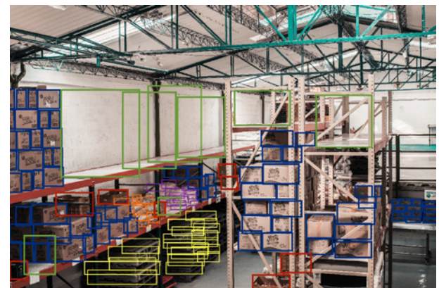
Figure 3 - Storage space recognition. Green bounding boxes indicate available storage spaces.
