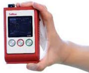
Figure 10: Soliton ZAO-S encoder for ultra-low latency h265. Transmitting over up to three 4G/5G LTE networks simultaneously.
